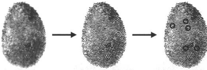
Figure 7.2: Automatic Extraction of Minutia
