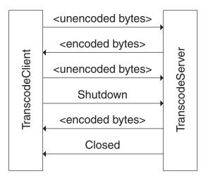
Figure 4.3: Transcode Server protocol termination.
