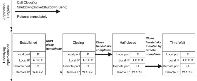
Figure 5.10: Closing a TCP connection first.
