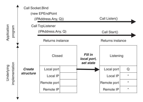
Figure 5.7: Server-side socket setup.
