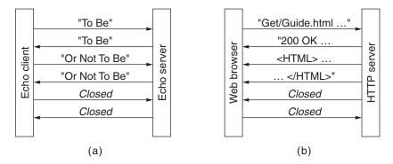
Figure 4.2: Echo (a) and HTTP (b) protocol termination.
