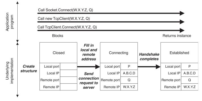
Figure 5.6: Client-side connection establishment.
