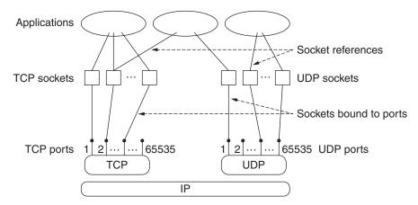
Figure 1.2: Sockets, protocols, and ports.
