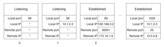
Figure 5.12: Demultiplexing with multiple matching sockets.
