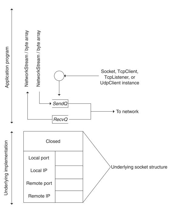
Figure 5.1: Data structures associated with a socket.
